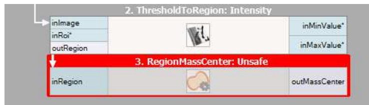
RegionMassCenter throwing a Domain Error on empty input region. The program execution is stopped.
