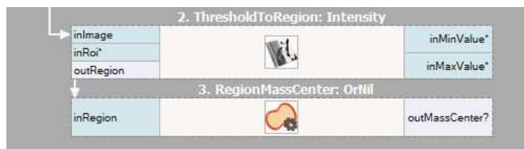
RegionMassCenter in the OrNil variant safely executed and introduces conditional processing on its output. Program execution continues.
