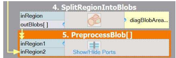
After optimizing: Only the final array is computed, reducing memory consumption. Please note that the macrofilter input is of Region, not RegionArray type.
