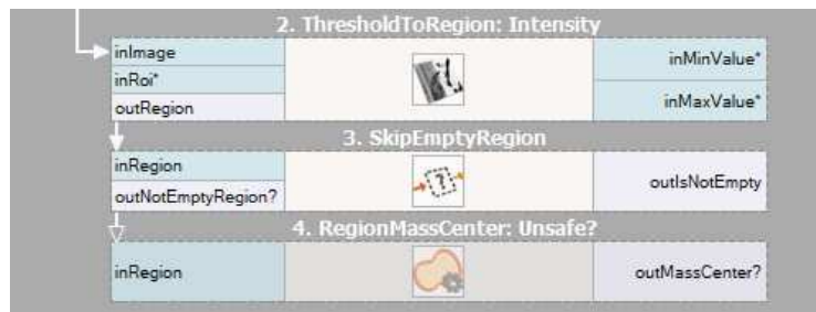
RegionMassCenter not being executed due to conditional processing introduced with SkipEmptyRegion . Program execution continues.
